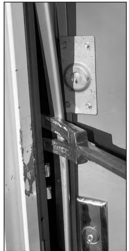
Figure #11--Push tool in sharply to force the door.
