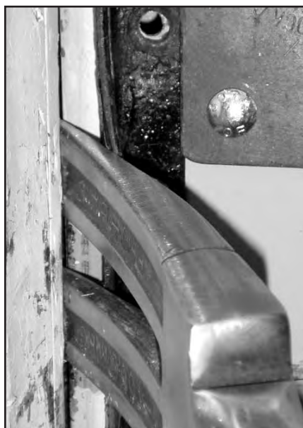
Figure #4--Push the tool toward the door slightly and drive in. Set the tips between the door stop and the door.
