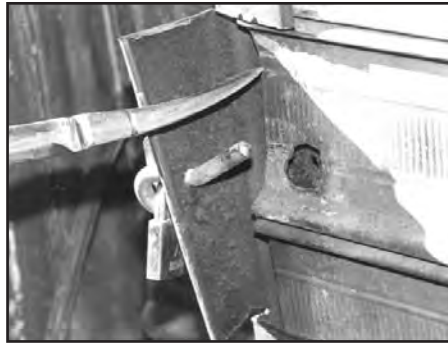
(Left) Bend the rail and pin out.
