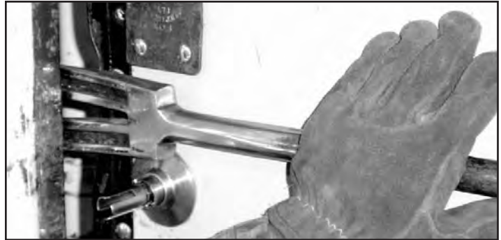
Figure #8--Push tool sharply toward door to force it.
